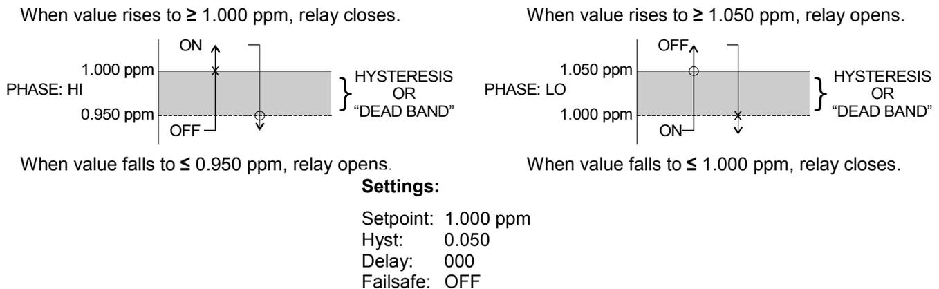
**Figure 18 - Control Relay Example**
