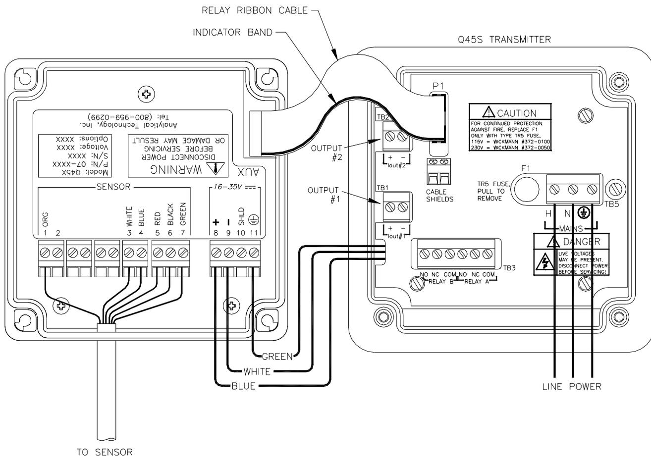
**Figure 14 - Sensor Connection**
