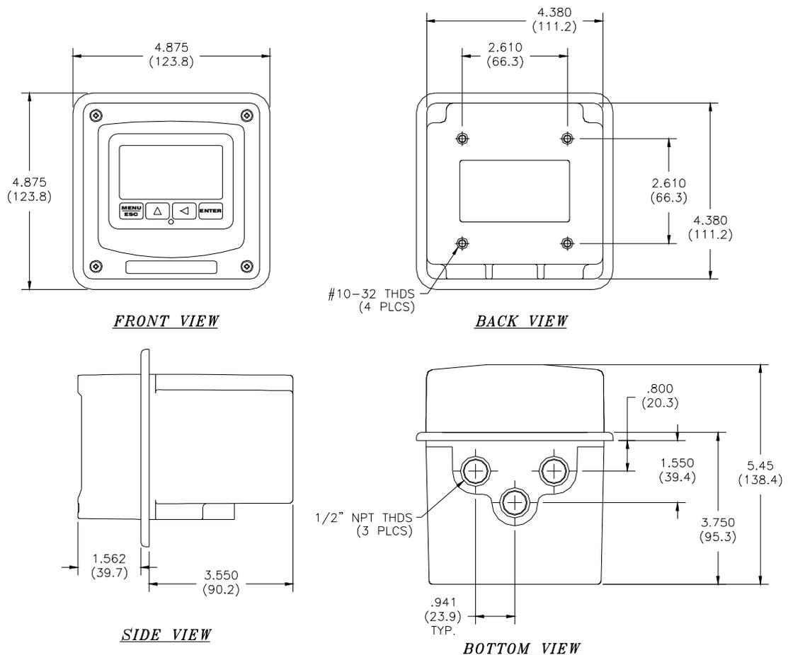
**Figure 2 - Q45 Enclosure Dimensions, AC Power**
