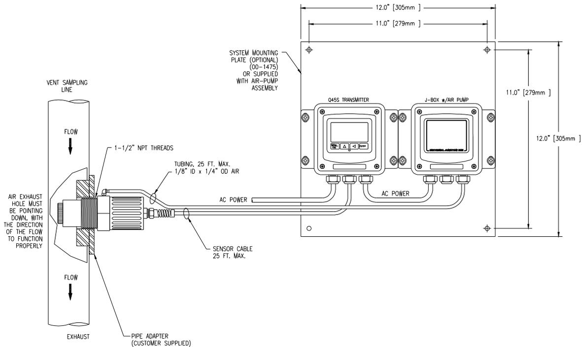
**Figure 1 - Wet H<sub>2</sub>S Typical System Diagram**
