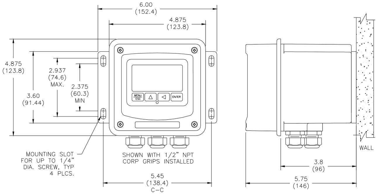
**Figure 5 - Wall Mounting Diagram**
