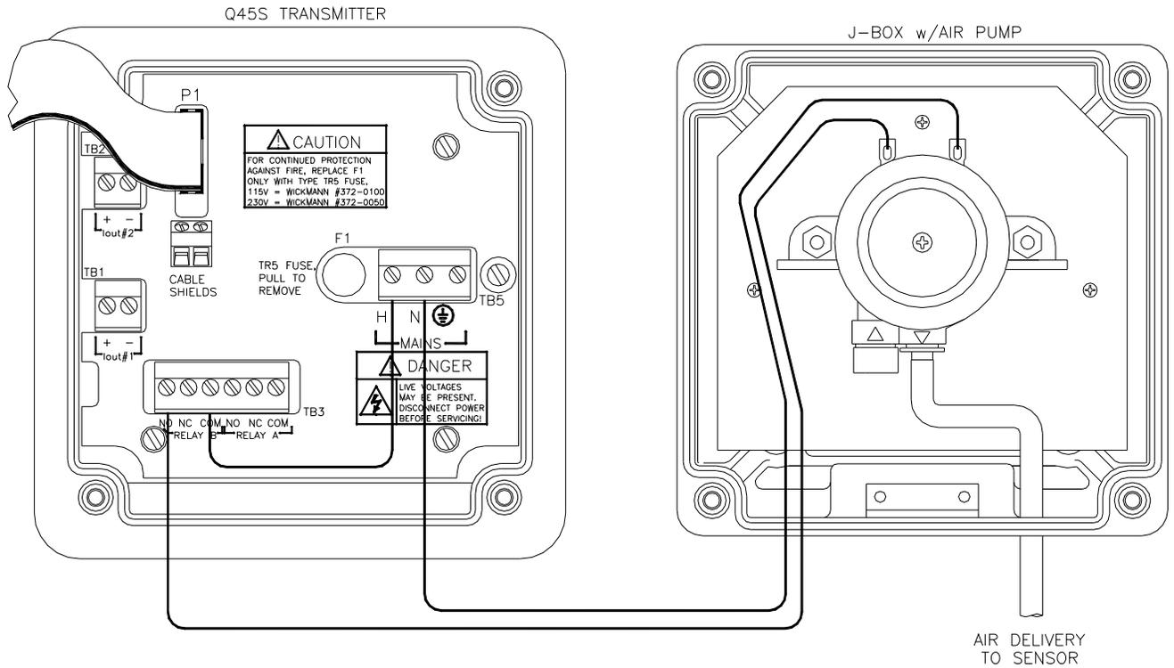
**Figure 12 - Pump Interconnect Connection**
