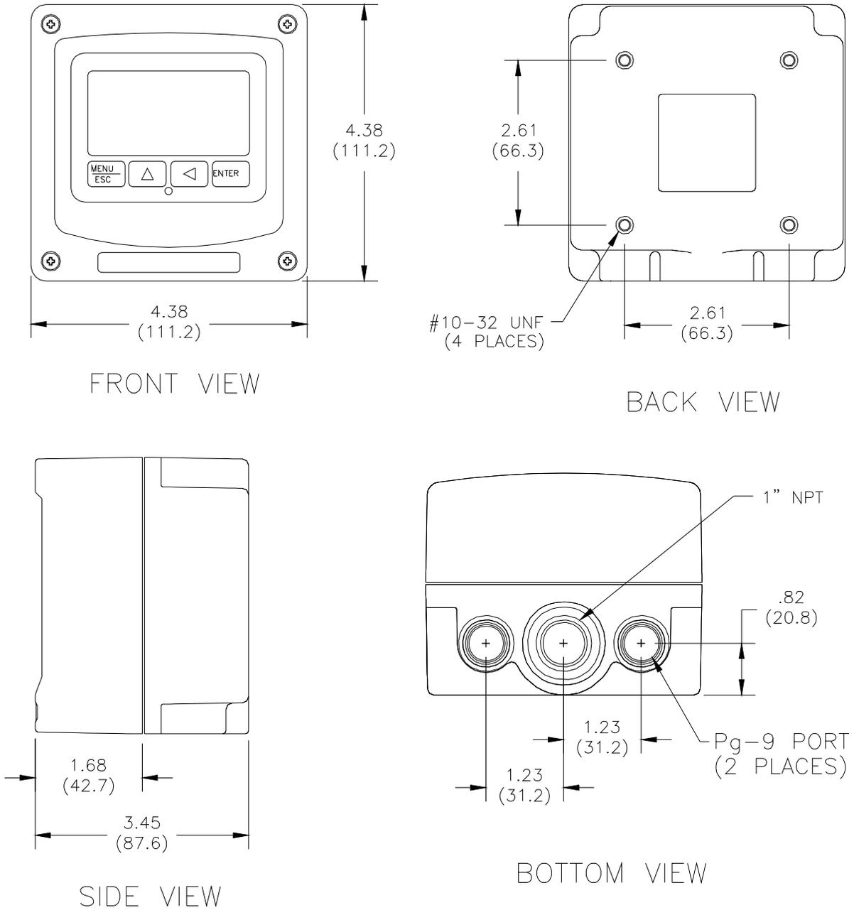
**Figure 3 - Q45 Enclosure Dimensions, Battery Units**
