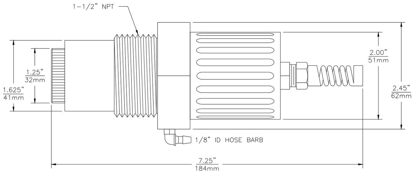
**Figure 9 - Duct Insertion Sensor Holder Dimensions**
