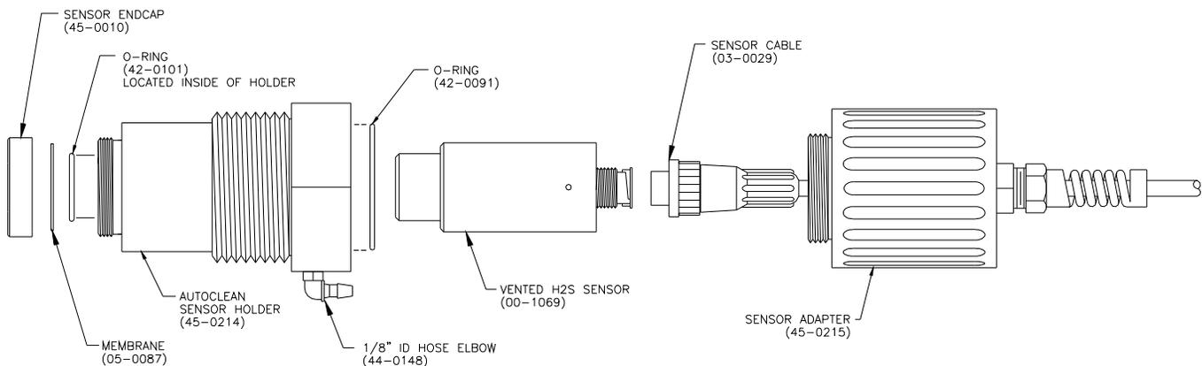
**Figure 10 - Duct Insertion Sensor Holder Exploded View**
