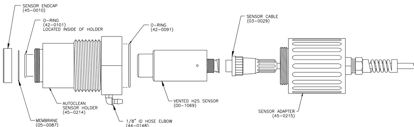
**Figure 7 - Duct Insertion Sensor Holder Exploded View**
