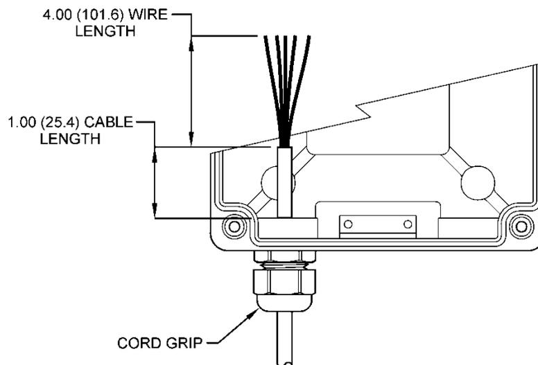
**Figure 9 - Sensor Cable Preparation**
