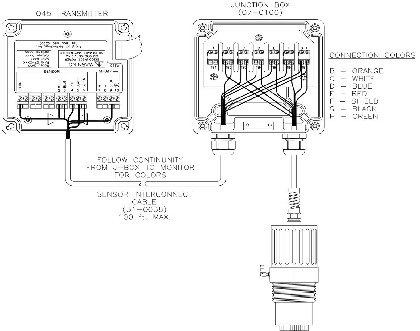
**Figure 10 - Junction Box Interconnect Wiring**
