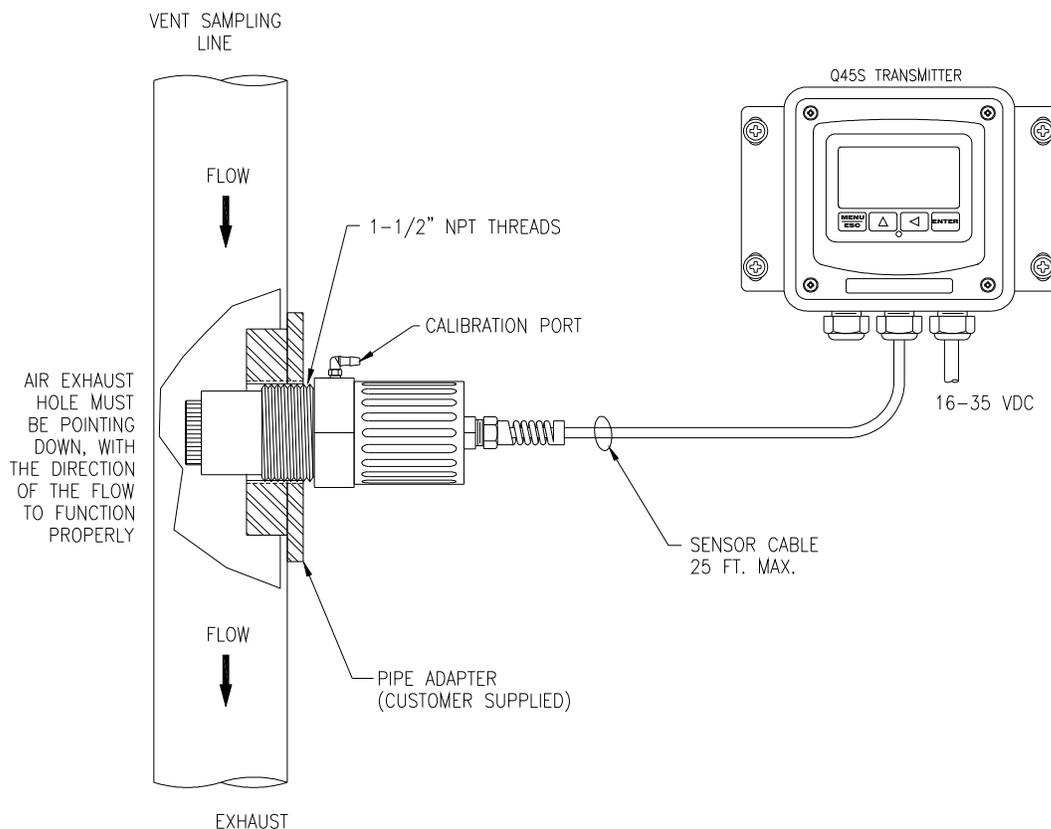
**Figure 1 - Wet H<sub>2</sub>S Typical System Diagram**
