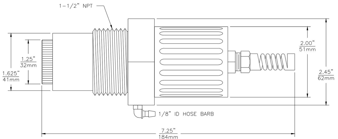
**Figure 6 - Duct Insertion Sensor Holder Dimensions**
