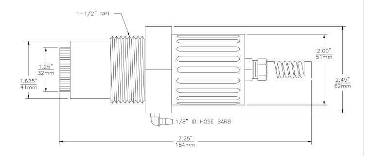
Figure 6 - Duct Insertion Sensor Holder Dimensions
