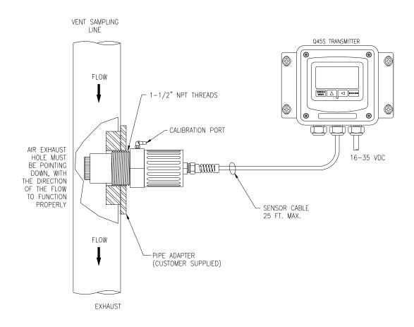
Figure 1 - Wet H2S Typical System Diagram
