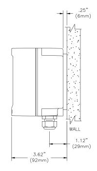
Figure 4 - Wall Mounting Diagram
