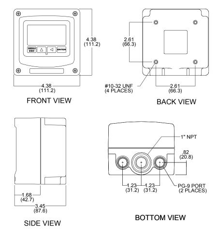
Figure 2 - Q45 Enclosure Dimensions, 2-Wire
