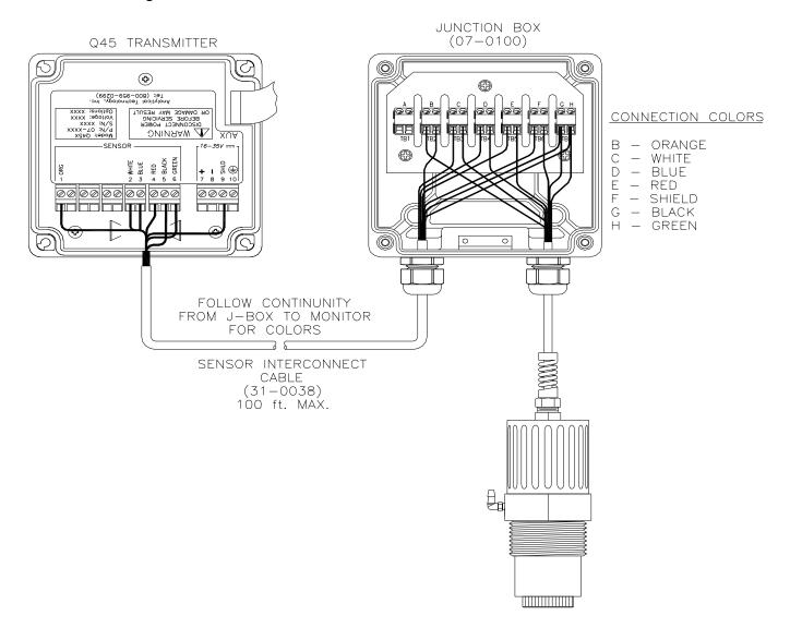
Figure 10 - Junction Box Interconnect Wiring
