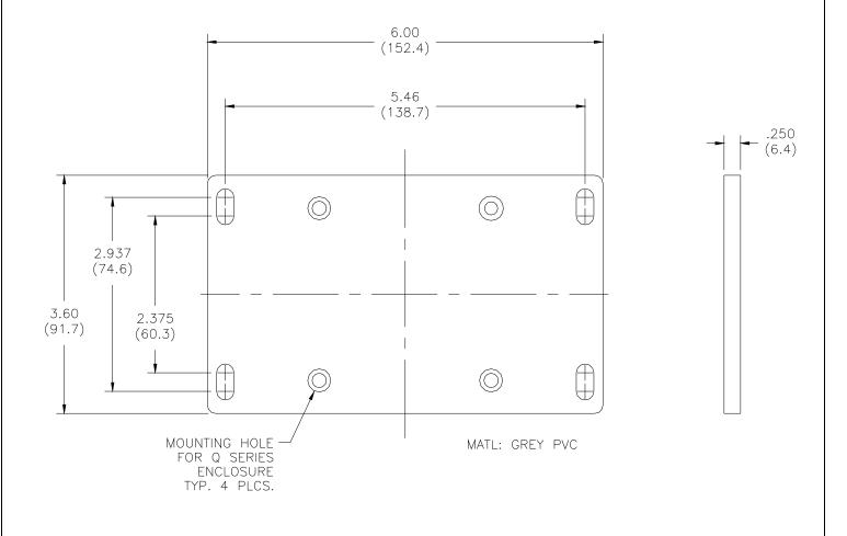
Figure 3 - Wall or Pipe mount Bracket
