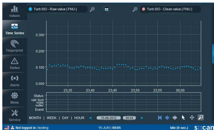
Fig. 14-1 Example for good turbidity measurement with expected noise levels in drinking water
