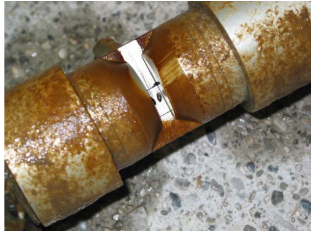
Figure 9: Efficiency of the automatic cleaning - the sensor is dirty but the measuring path is free of fouling
