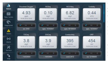
The <u>Values</u> screen provides a detailed overview of the last parameter results as well as status information from all configured sensors.
