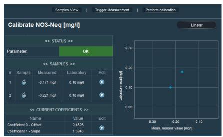
Pushing <u>Perform Calibration</u> starts the selected calibration procedure with the two samples as displayed (select <u>Samples</u> <u>View</u> for checking graphically). When calibrating is finished a user message will inform if it was successful. In case of an error the reason will be displayed to the user in red letters (e.g. Please enter at least lab values for 2 samples).
