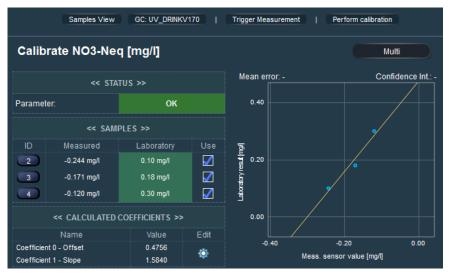
In the <u>Samples</u> area the ID and values of all stored samples valid for the respective sensor / parameter are displayed. Pushing the ID number switches to the respective <u>Sample list</u> results as explained in chapter 6.3.3.
