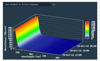
Besides the standard two-dimensional view it is also possible to show fingerprints from one spectro::lyser in a three- dimensional graph which provides a good impression of quality developments.
